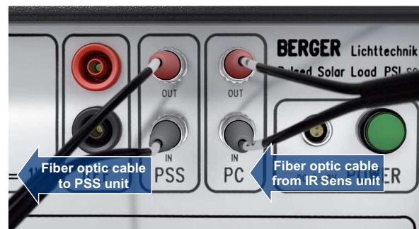
Figure 5 | Fiber optic cable connections at PSL unit
