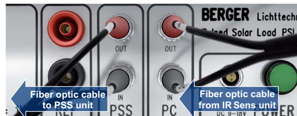
Figure 10 | Fiber optic cable connections at PSL unit
