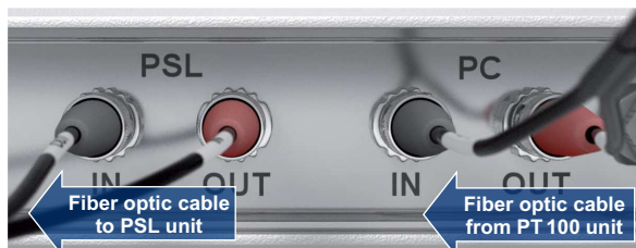
Figure 9 | Fiber optic cable connections at the IR Sens unit
