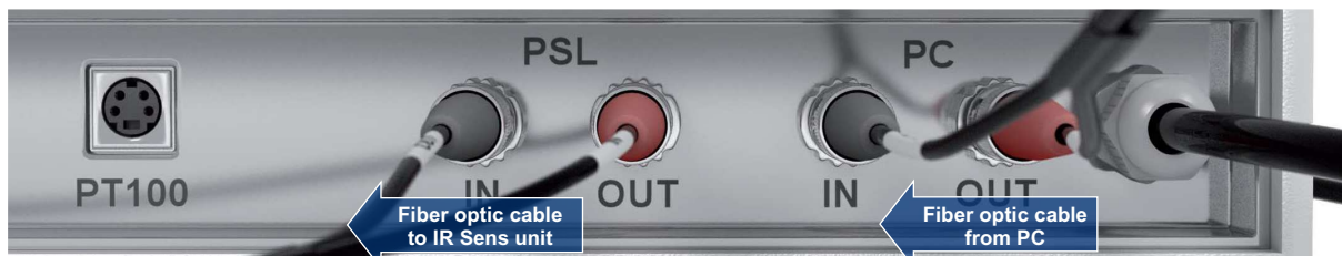
Figure 8 | Fiber optic cable connections at the PT 100 unit
